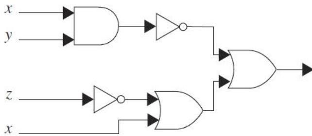
The output of the circuit is  $\overline{xy} + (\overline{z} + x)$
