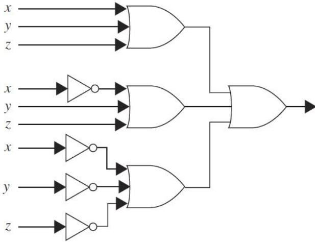
The output of the circuit is  $(x + y + z) + (\bar{x} + y + z) + (\bar{x} + \bar{y} + \bar{z})$
